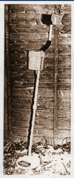
than Disc 1, and is brought into operation by pressing and holding down the 'Disc 2 Push Select Button'. The purpose of this 'dual channel discrimination' is to give the user more information on a target and thus enable a decision to be made as to whether the target should be dug or ignored.
