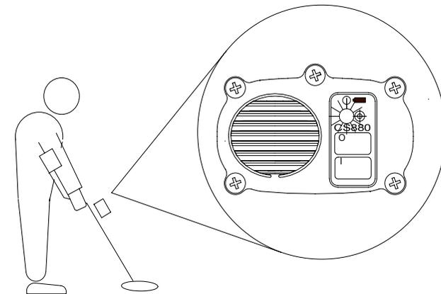
Detection of a metal cover is indicated by an audible pitch increase and target light brightness increase. Small metal targets are ignored.
