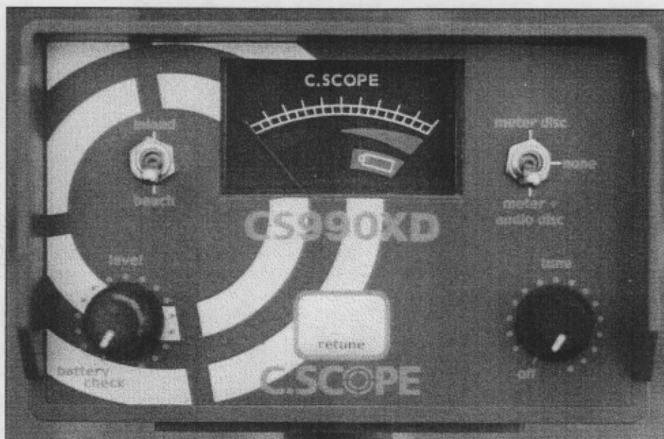
Fig.2. The CS990XD's control panel.
