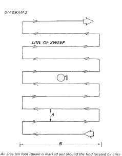
An area lett floot square is marked out around the find located by crisscross search. This is then divided into strips which are carefully searched. Distance A = width of the detector's pick-up area. Distance B = length of a comfortable sweep.
